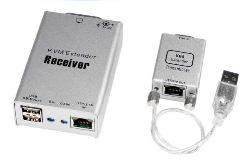
The Single PC, Single Access KVM Extender Kit is perfect for any type of installation where the console needs to be in a conveniently accessible location, but the computer system to reside in a long distance place away from dust, and harsh environmental influences. The K30460US-15 or K30460US-30 CAT 5 KVM Extender Kit, which effectively extends PC KVM (USB Keyboard, Video, USB Mouse) control to the Console Receiver.
